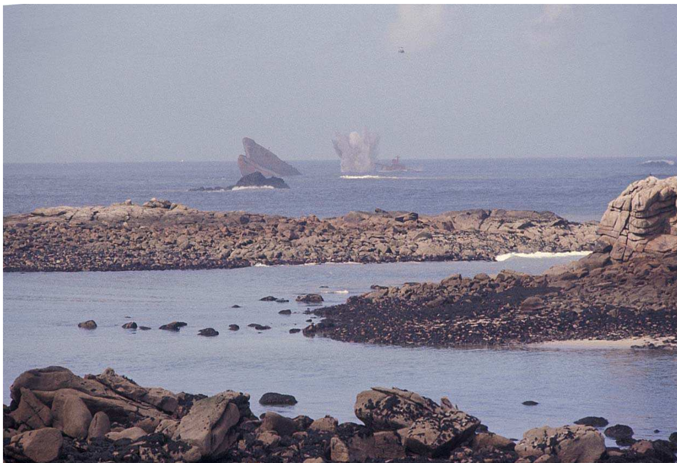
Figure 3.2. On 16 March 1978, the oil tanker Amoco Cadiz, transporting 227,000 tonnes of crude oil, suffered a failure of her steering mechanism, and ran aground on Portsall Rocks, on the Breton coast. The entire cargo spilled out as the breakers split the vessel in two, progressively polluting 360 km of shoreline from Brest to Saint Brieuc. This was the largest oil spill caused by a tanker grounding ever registered in the world. The consequences of this accident were significant, and it caused the French Government to revise its oil response plan (the Polmar Plan), to acquire equipment stocks, and to impose traffic lanes in the Channel. The photo shows the wreck of the Amoco Cadiz while being bombed by a helicopter to release the remaining oil from its holds. © CJ Camphuysen
